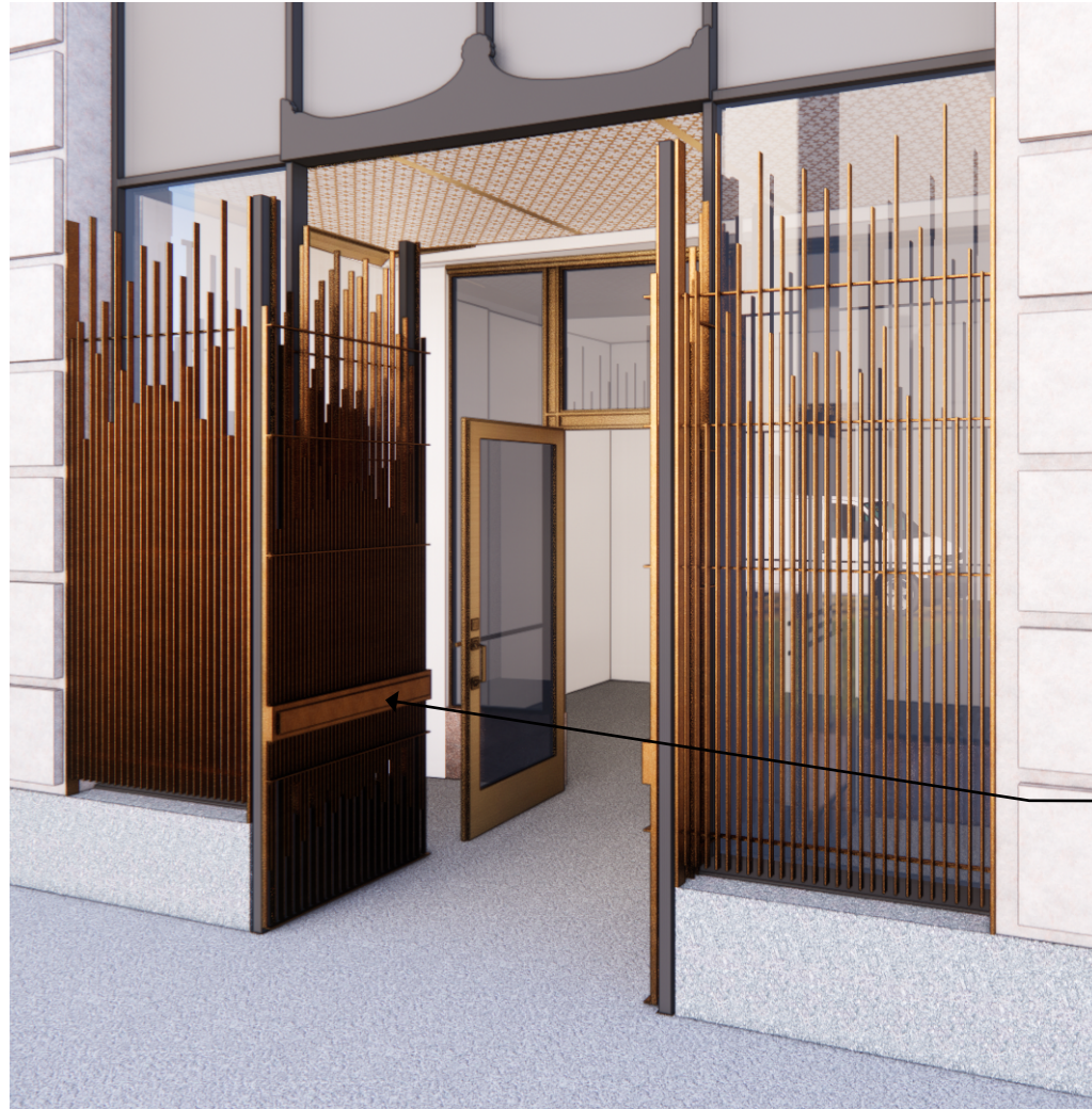
EMERGENCY DOOR HARDWARE
