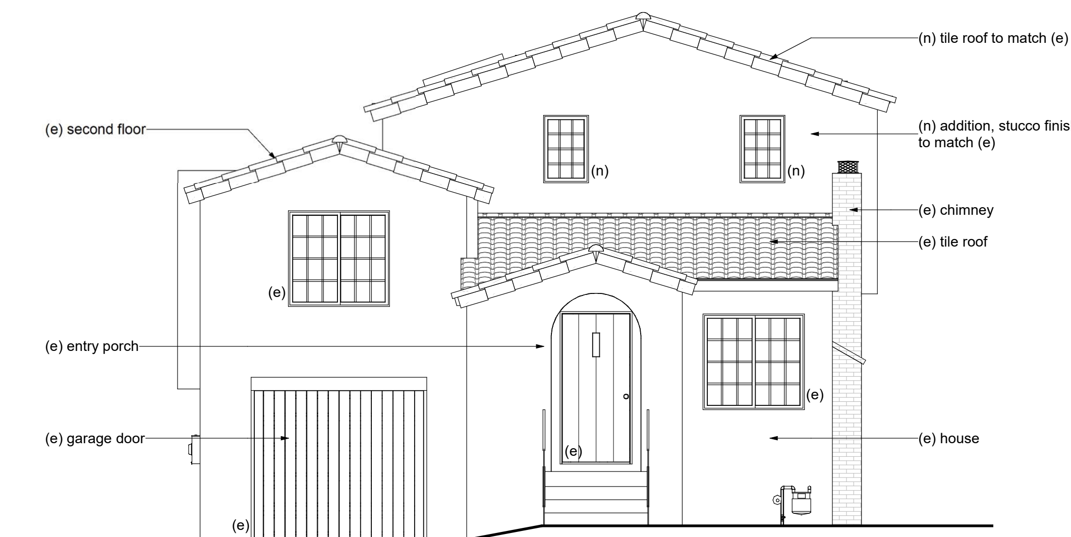
1 Proposed North Elevation - Front AUP Modification
