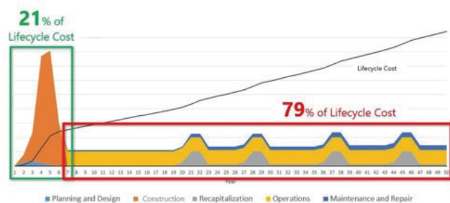
▲ Figure 7: Typical costs to manage a facility from construction to disposal, from RTD Denver
