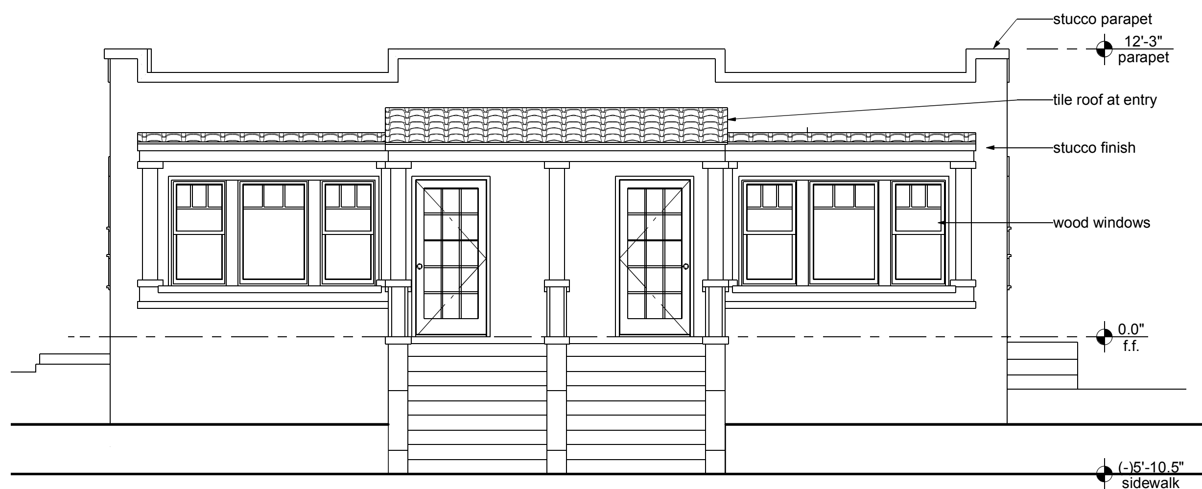
2 Existing West Elevation - Front
