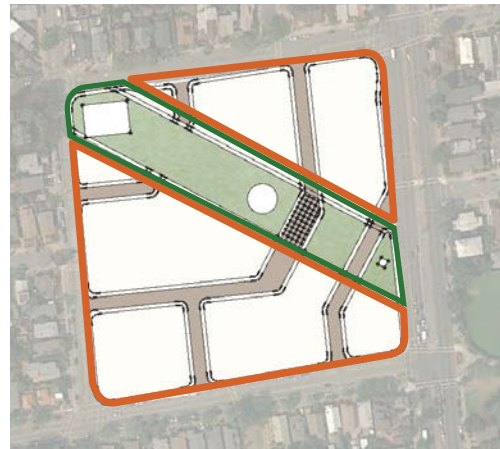
█ BART Easement (approx. 3 acres) █ Developable Area (approx. 5 acres) Total Site Area = approx. 8 acres
