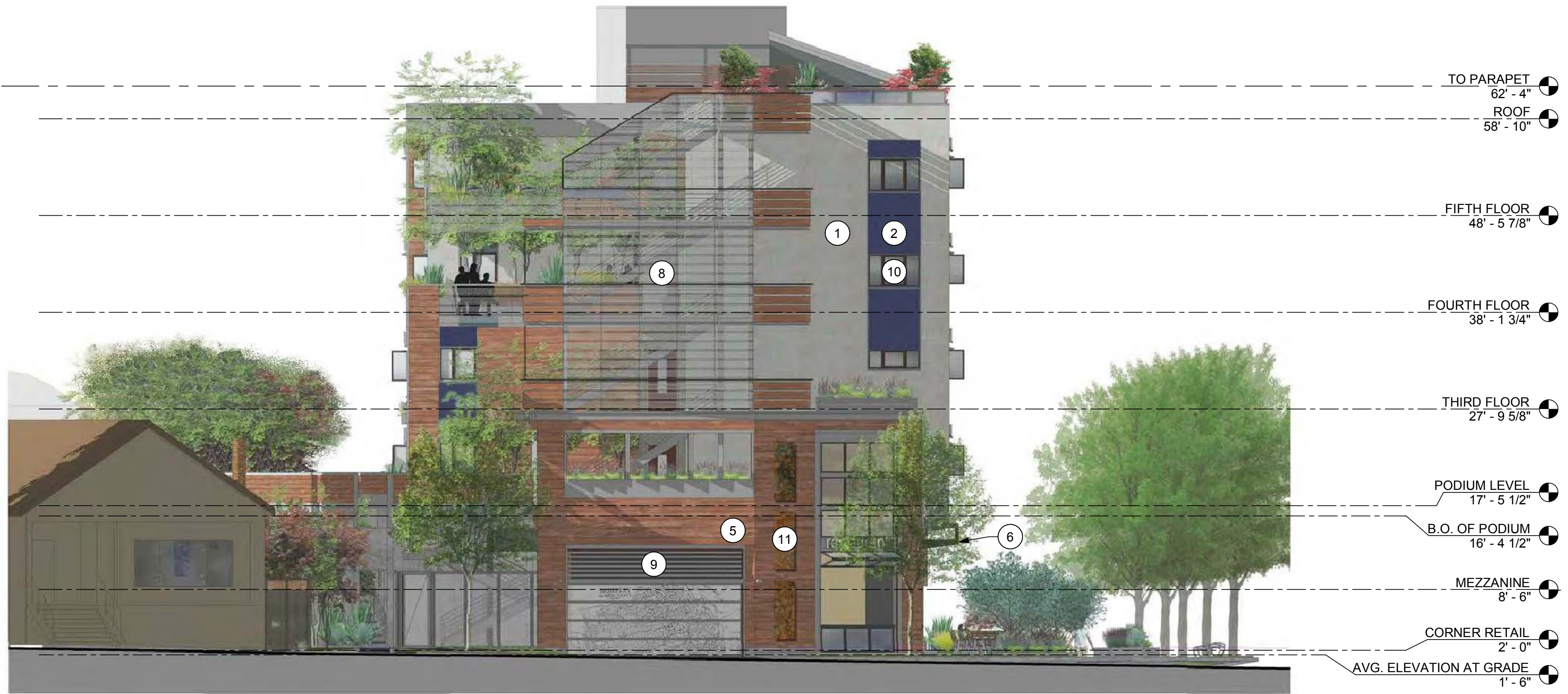
2 EXTERIOR ELEVATION - NORTH 1/8" = 1'-0"
