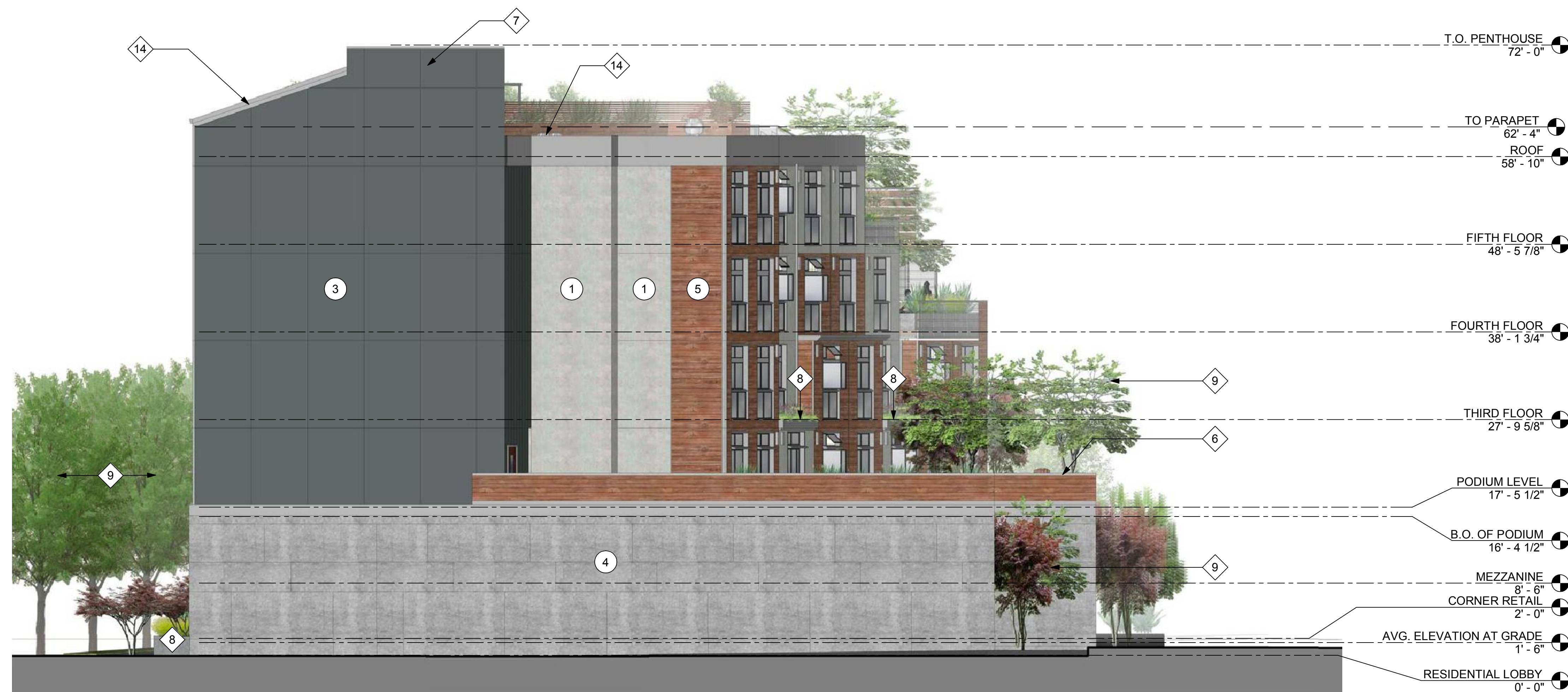
2 EXTERIOR ELEVATION SOUTH 1/8" = 1'-0"
