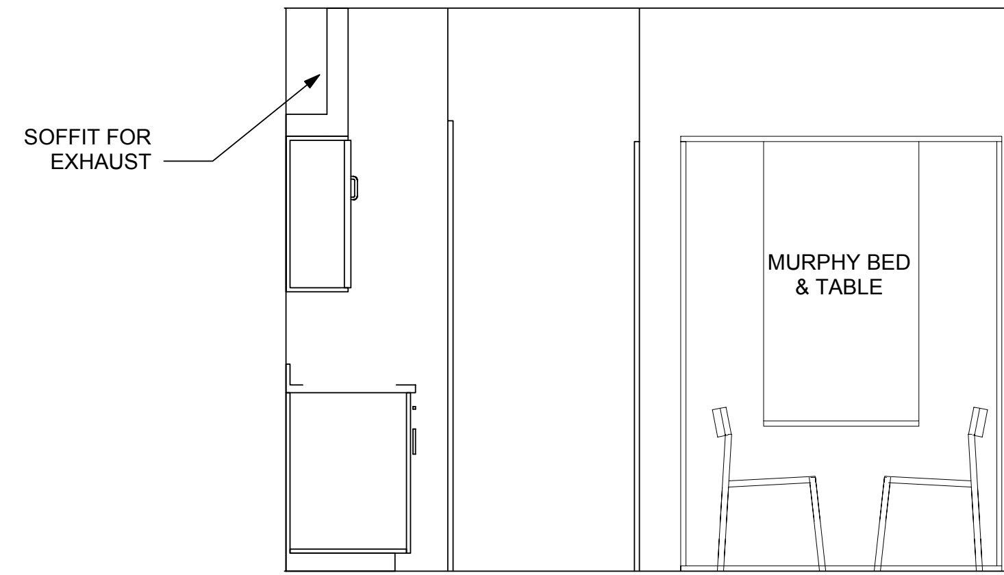
6 WEST ELEVATION OF UNIT A2 1/2" = 1'-0"
