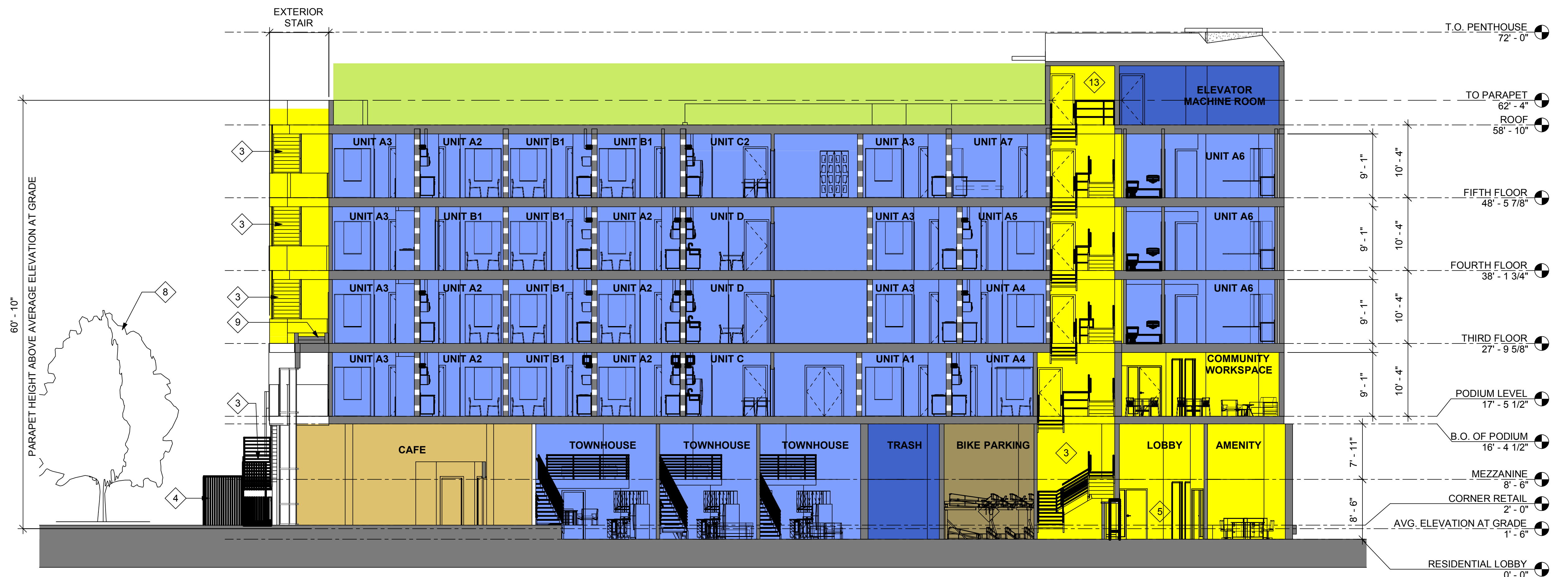
① LONGITUDINAL SECTION THROUGH UNITS 1/8" = 1'-0"
