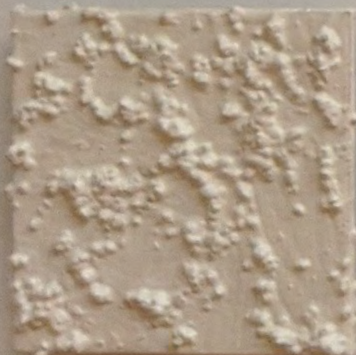
MONUMENT BASES 0.063" ALUMINUM SHEET PAINTED PPG BRP 1501: ACRYLIC URETHANE PPG10241-1 "OFF WHITE" MEDIUM STUCCO FINISH
