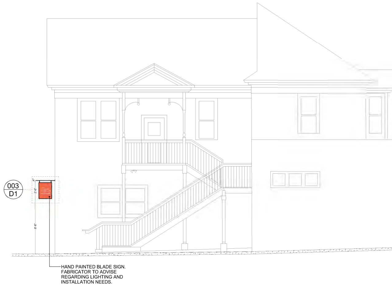
2 SIGN LOCATION - SIDE ELEVATION A
