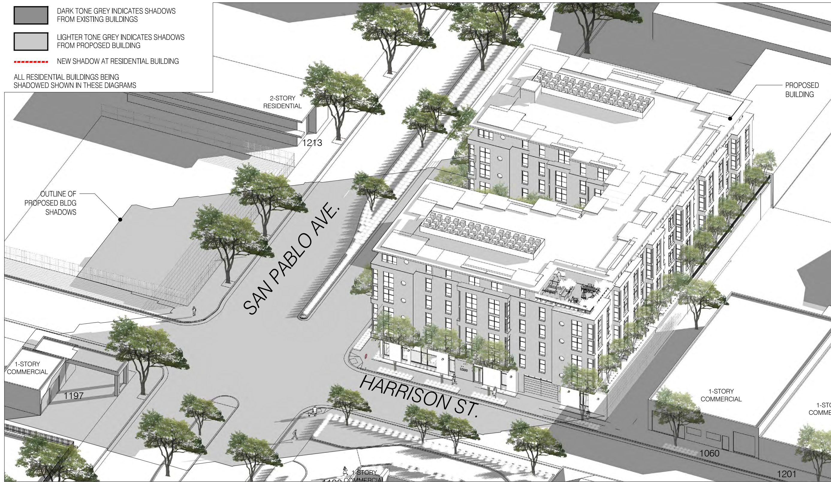
4 SHADOW STUDY AXONOMETRIC - DEC 21: 2-HRS BEFORE SUNSET NTS
