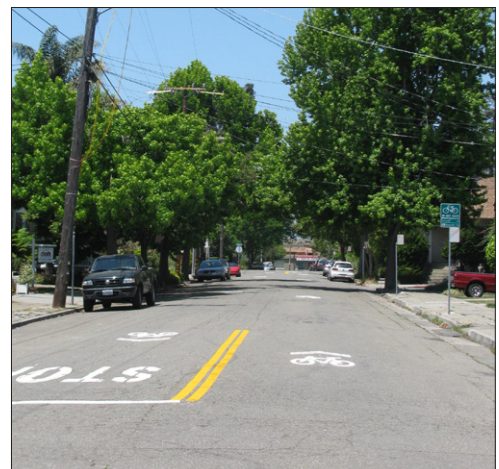
Figure 5: 50 ft double centerline
