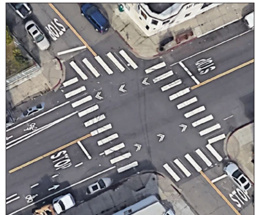
Figure 3: Intersection chevron markings, 38th Ave and Brookdale Ave
