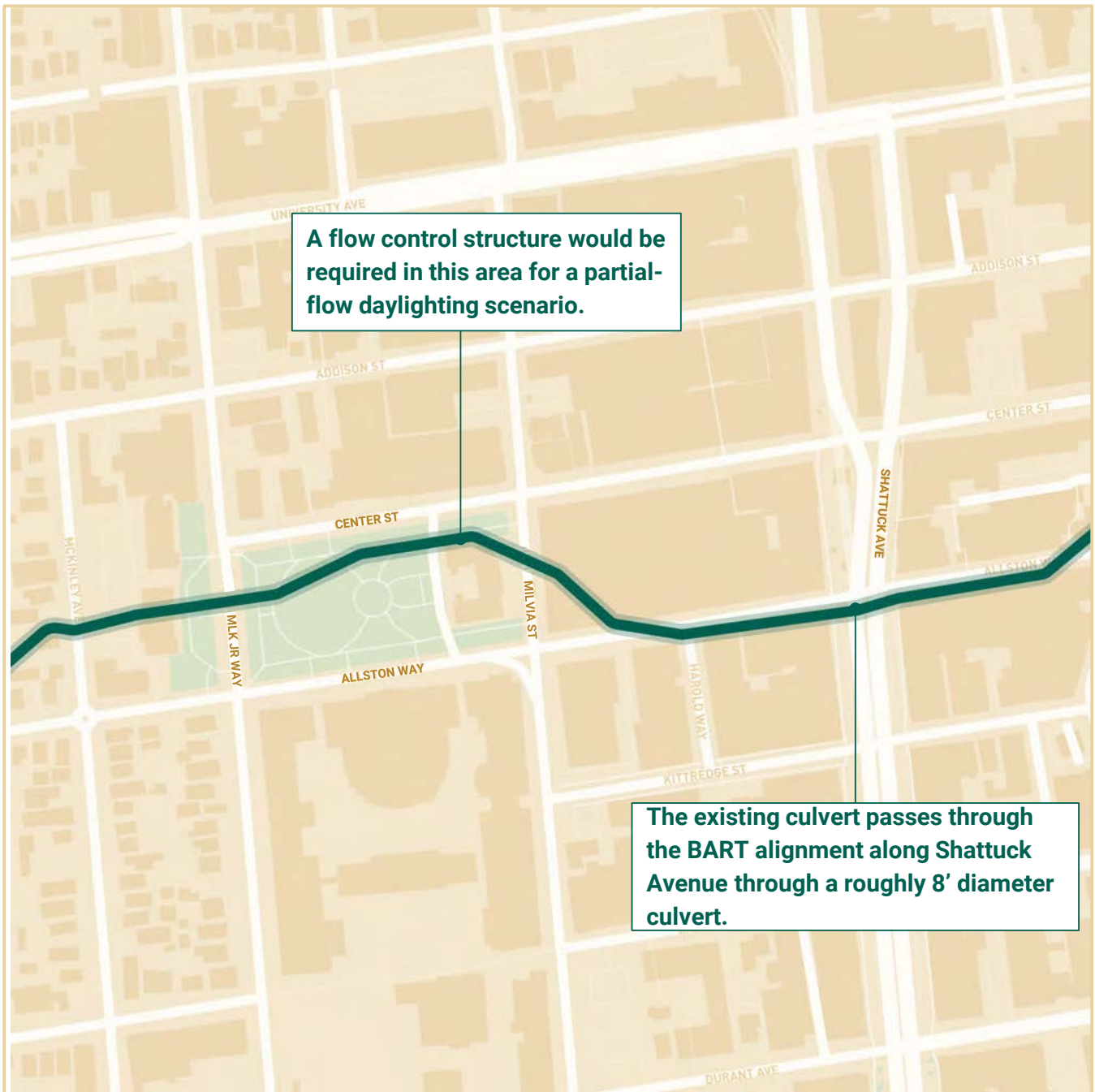
Existing Strawberry Creek culvert location in Downtown Berkeley (based on Wolfe Mason Study From 1999)
