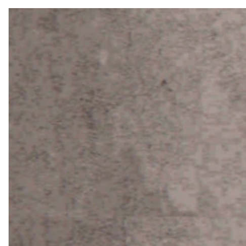
INTEGRAL COLOR STUCCO STEEL HARD TROWEL FINISH
