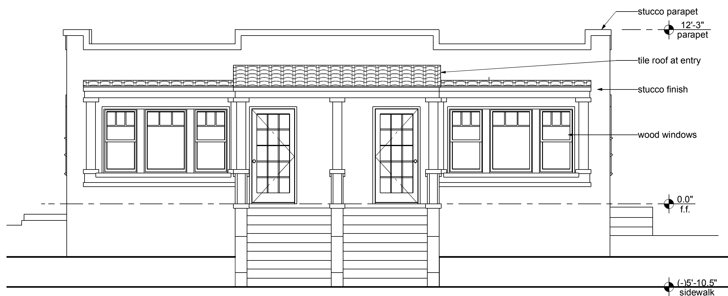
2 Existing West Elevation - Front
