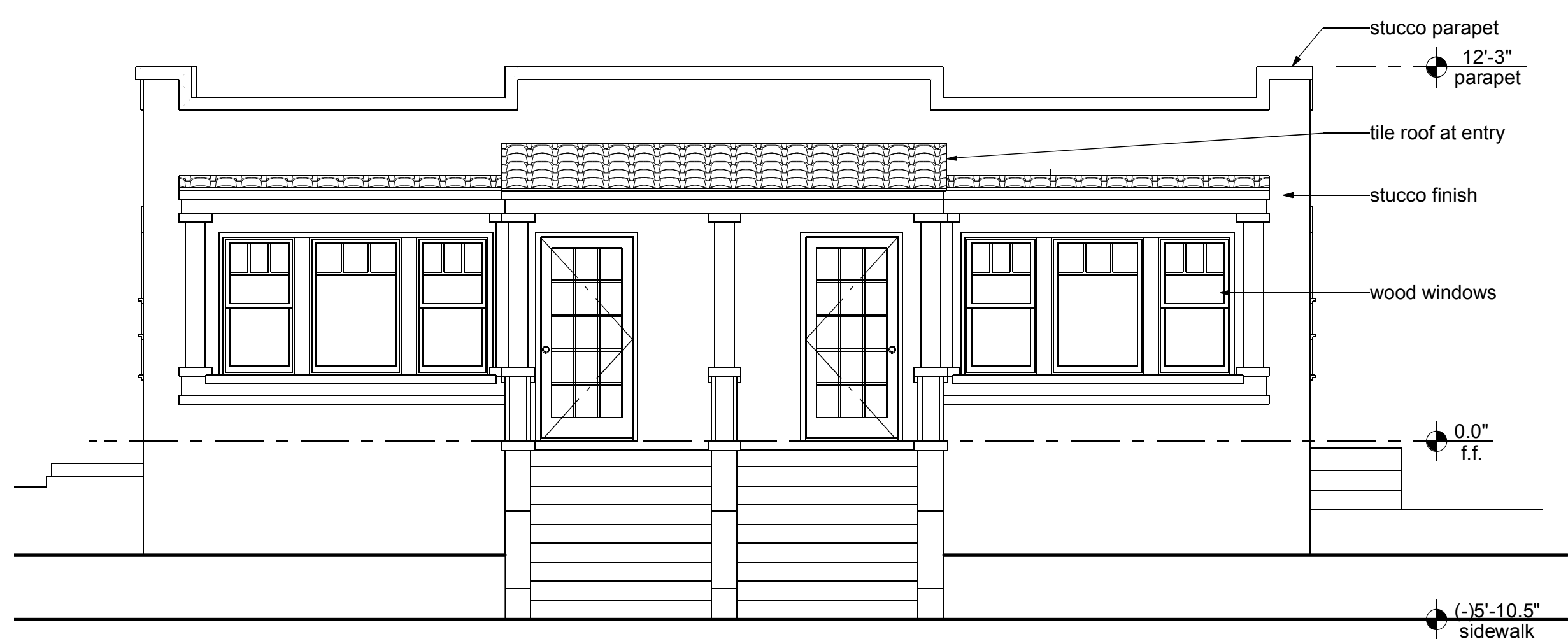
2 Existing West Elevation - Front
