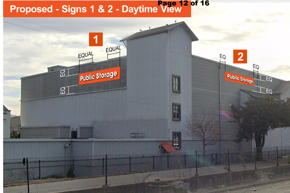
Proposed - Signs 1 & 2 - Daytime View NORTHWEST CORNER ELEVATION BLDG C - STORAGE NEW REVERSE CHANNEL LED HALO-ILLUM'D LETTERS ON B/G PANELS ALLOWED SF: 2000 AGGREGATE PROPOSED SF: 171.1 SF (N. ELEV.) / 130.4 SF (W. ELEV.)
