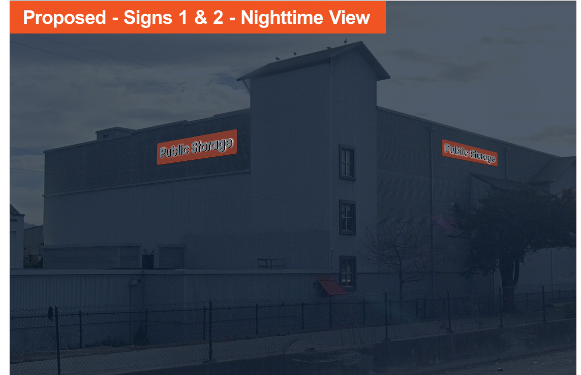
Proposed - Signs 1 & 2 - Nighttime View HALO-ILLUMINATED REVERSE PAN CHANNEL LETTERS ON A B/G PANEL - SIMULATED NIGHT VIEW
