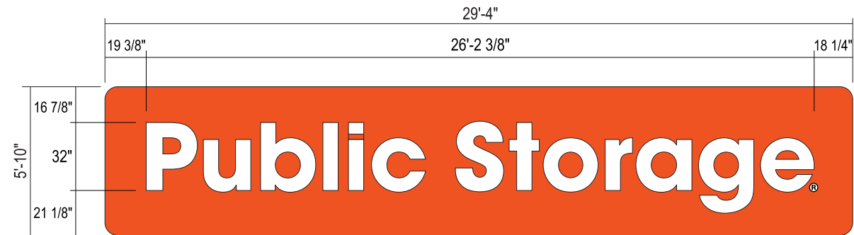
1 CUSTOM - HALO ILLUMINATED REVERSE CHANNEL LETTERS - B/G PANEL SCALE: 3/16"=1'-0" LETTER AREA (BOXED) - 93.0 SF PANEL AREA - 171.1 SF
