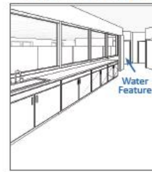
Security glazing allows staff to view the stabilization room through two-way windows (clients cannot see into the office) for monitoring and observation.
