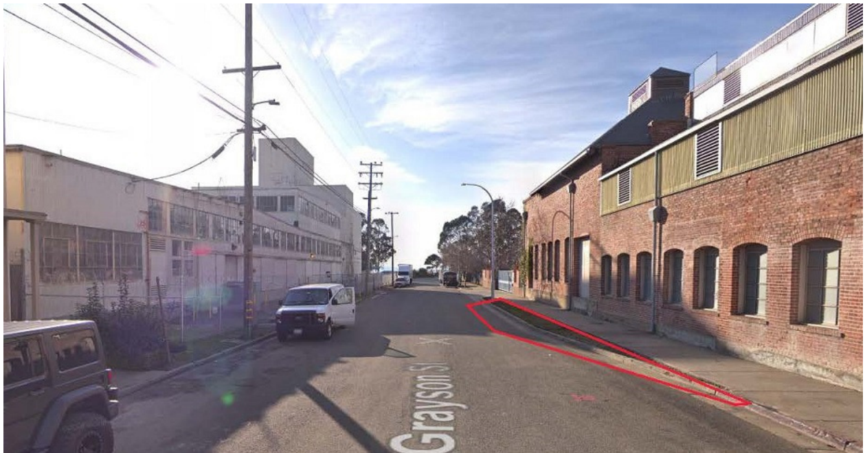
Figure 30 – Extension and retrofit of existing sidewalk planter strips into bioretention features may be feasible on Grayson Street between Seventh Street and the UPRR ROW.
